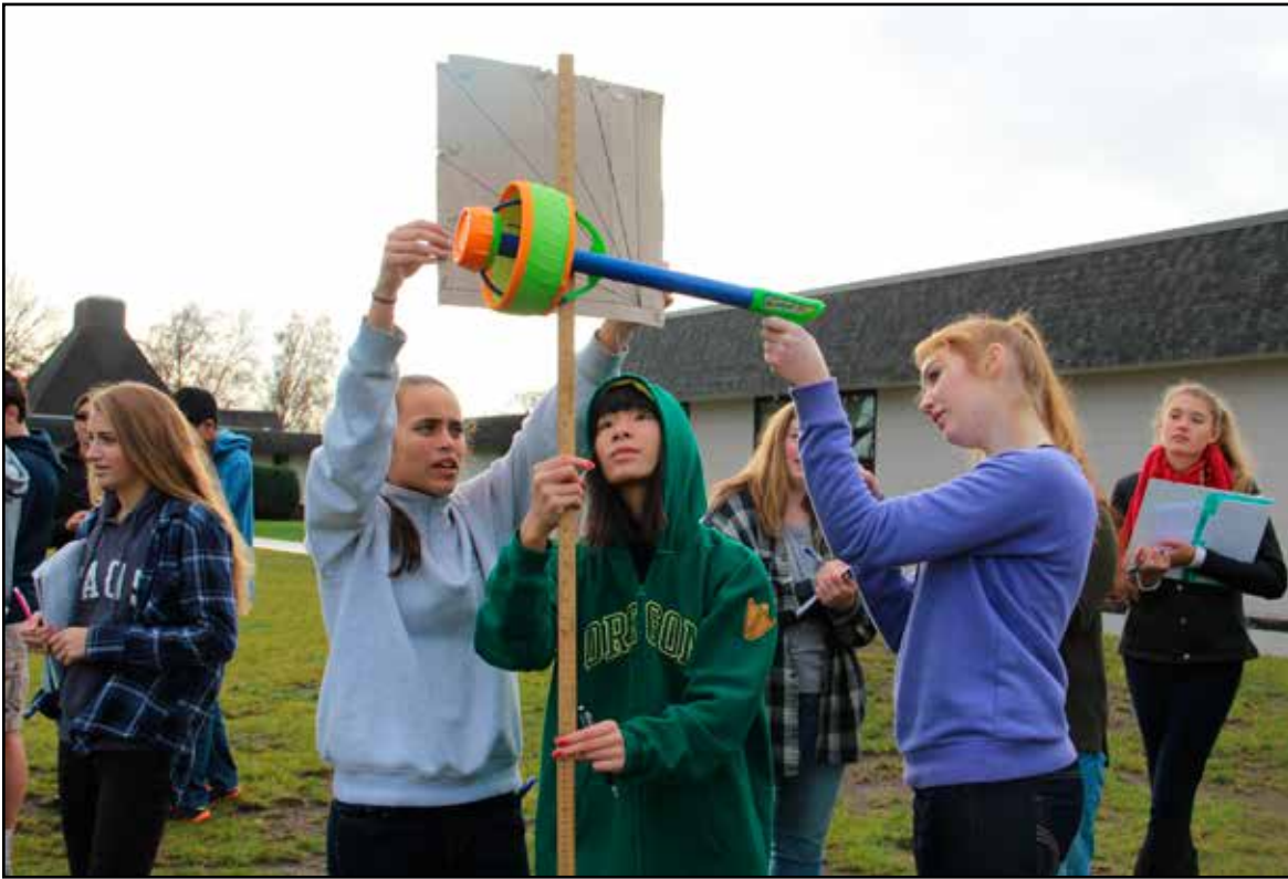
Norman Miller's freshmen physical science students measure the angle at which a projectile will be launched outside during class on Thursday. The freshmen spent the block period launching projectiles to learn about how the height and angle of an object affects how far the object will travel. This is Miller's first year as a teacher at Marist. Photo by Madi Potter
