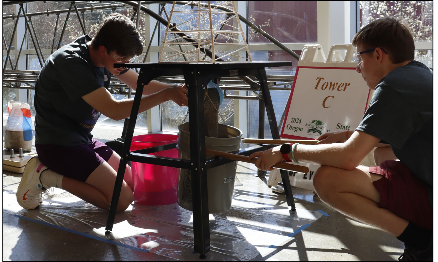
Sophomore Bruce Clark and Senior James Smythe test the load capacity of their wood tower. Photo by Elizabeth Tucker '24
